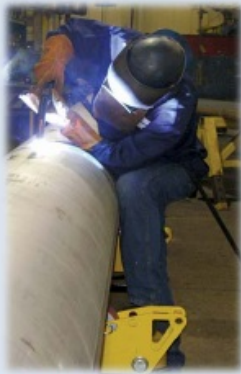
From left: HD2L-100/150 roll welding large bore pipe, AC controller, forward/reverse foot switch, HD2L-100/150 setup
